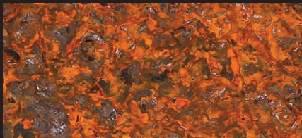
Without corrosion protection treatment
